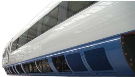
Pre-filtration of air intake filtration for air conditioning systems
