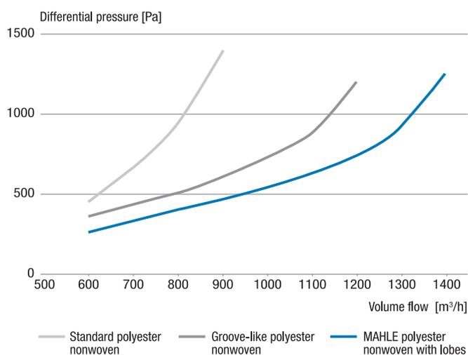
*Clear performance advantage using the ridges technology: greater volume flow at a lower differential pressure.*
