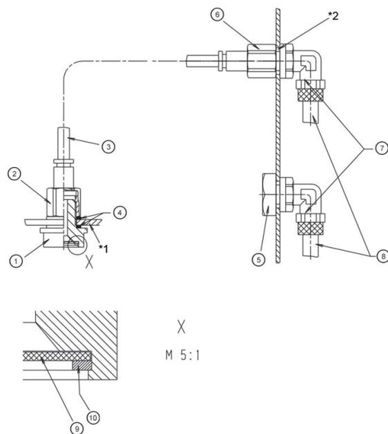
\*1 = bore  $\varnothing$  13.5 mm in the filter plate
