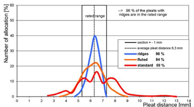
Comparison of the pleat allocation between the pleat distance controls of fluted filter media and with or without the MAHLE technology of ridges
