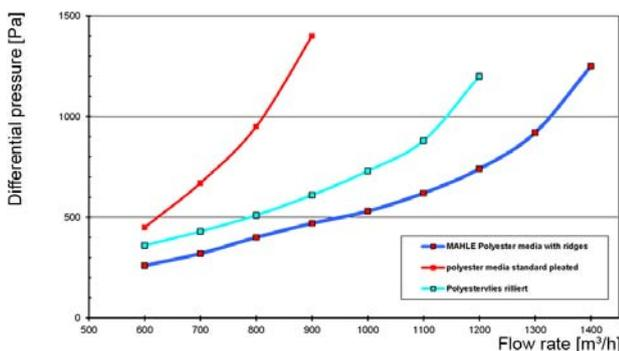
Comparison of differential pressure development on load with fluted filter media, with and without the pleat distance control with the MAHLE technology of ridges
