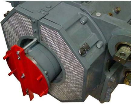
Pre-filtration of air intake filtration for electrical engines
