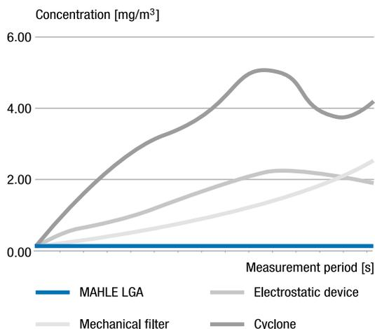
*Low emissions values substantiate the consistently high retention efficiency of the MAHLE LGA series (in comparison with conventional separators).*
