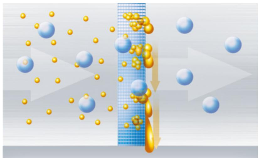
*Higher performance, longer service life, and lower maintenance costs thanks to the coalescer filter principle: the oil mist “coalesces” into larger droplets, which are efficiently separated.*
