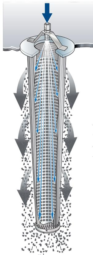
*The optimized multijet nozzle provides for highly efficient cleaning with low compressed air consumption.*
