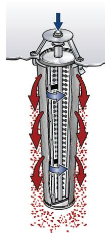
With the rotation wing a gentle cleaning is possible, which extends the life of the filter cartridges remarkably.
