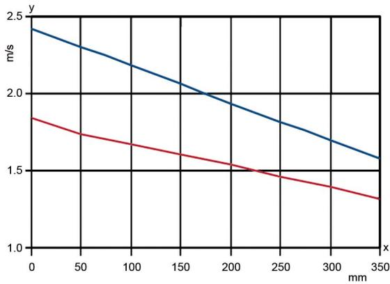
The conical design of the cartridge shows a high reduction of the upstream velocity in the area of the bottom end cap. Through it the element is much better to clean off, especially in use of light dust. The dust can sediment better.
