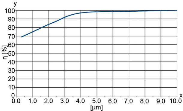
Filtration efficiency: > 98 % at 5 μm
