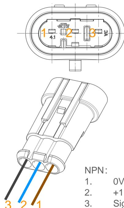
**Dia. 18.2** Divider Monitoring Sensor Wiring Connection
